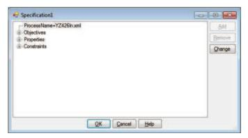
Note that the Process has been filled in already because the ReferenceRun contains only one Process. If the ReferenceRun had contained multiple Processes, you would have been required to select the Process node, click the Change button and select the Process for this Specification. Click the Objectives node and click the Add button. The Objective Dialog is displayed.
