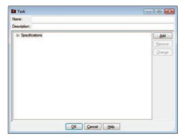
Type Maximize BMEP as the Task name and Virtual Engines Task as the description. Click the Specifications node and click the Add button to display the Specification dialog.
