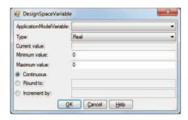
Select EXP1.S(4).EntranceDia as the ApplicationModel variable and type .02 as the Minimum value and .05 as the Maximum value. Note that all values are expressed in meters because the Virtual Engines files store all length values in meters.
