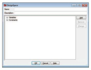
Type Vary Exhaust Section 4 Length and Diameter as the DesignSpace name and Virtual Engines DesignSpace as the description. Click the Variables node and click the Add button to display the DesignSpaceVariable dialog.
