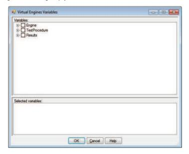
The Virtual Engines Variables dialog displays a tree view of the Engine, TestProcedure and Results and is similar to the tree view that the Virtual Engines Design application or the Automated Design Knowledge Engineering Interface application. Expand the Engine, Pipes, EXP1, Sections and Section(4) nodes. Click the checkboxes on the EntranceDiameter and Length nodes. Expand the Results node and click the checkbox on the BMEP node. Your Virtual Engines Variables dialog should look like this:
