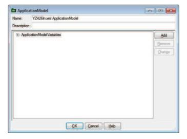
Note that the Virtual Engines interface has supplied a name for the ApplicationModel. Right-click the ApplicationModelVariables node on the ApplicationModel dialog and select Add from the menu to display the ApplicationModelVariable dialog. Scroll to the bottom of the list of VariableSpecifications. Click Exp1.S(4).EntranceDia. Shift-click Exp1.S(4).Len and BMEP. The dialog will look like this:
