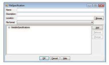
Click the "Browse" button and select YZ426In.xml from the Virtual Engines or Automated Design DATA folder as the location. The FileSpecification dialog will fill in the FileSpecification name, location and format for you. Right click on the VariableSpecifications node in the FileSpecification dialog and select Add from the menu. The Virtual Engines Variables dialog is displayed.
